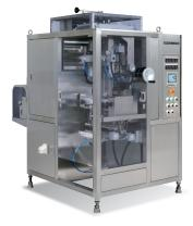
"Twin Pack" or "4 side seal" Pouch Bag Filler for liquid / viscous sachets. It is possible to fill up to 1L without head space. (2 heads are also possible). A servo motor is installed in the seal mechanism to improve seal strength and seal quality.
