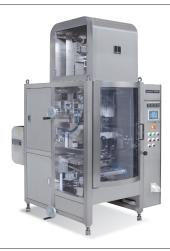
This is a filling and packaging machine designed for "3 side seal" small pouches for liquids and viscous product. It is possible to pack up to 60 ppm with 1 head and 120 bags with 2 heads. Servo motors are installed in the seal mechanism to improve seal strength and quality.
